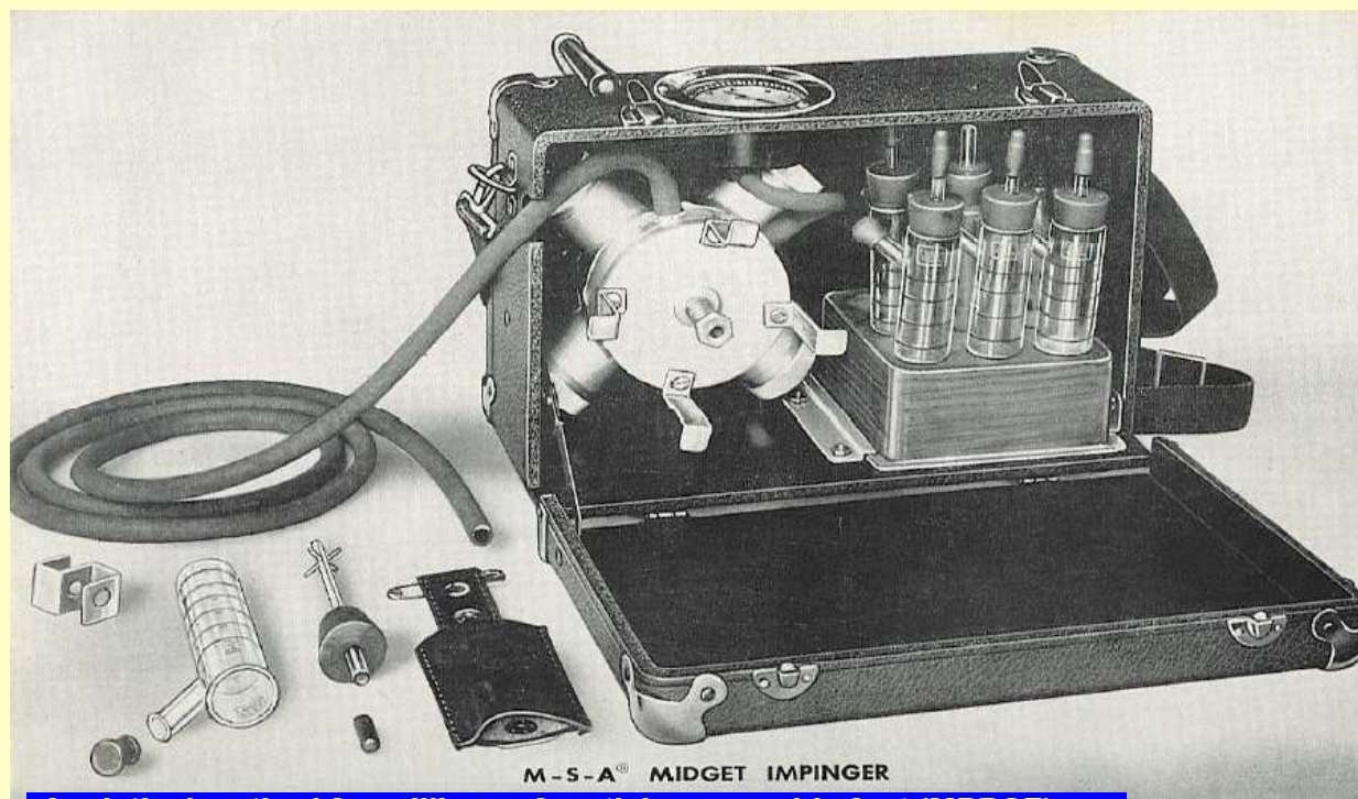
Analytical method for millions of particles per cubic foot (MPPCF) Standard procedure for sampling and counting dust – adopted by the ACGIH in 1942
